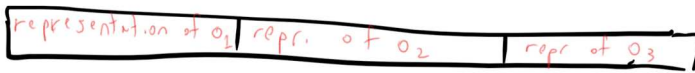
Figure 2.4: If we have a prefix-free representation of each object then we can concatenate the representations of k objects to obtain a representation for the tuple (o_1, \dots, o_k) .
